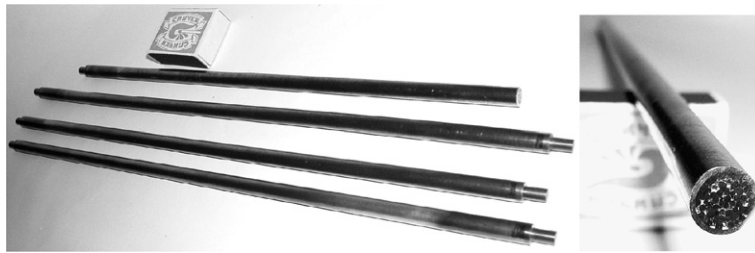
Fig. 6. Appearance of fuel elements 9.15 mm in the diameter produced by capillary impregnation method [2].
